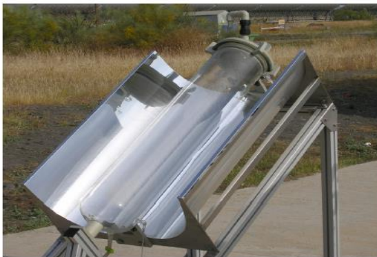
Fig.7 A compound parabolic collector with borosilicate glass absorber tube (Nalwanga et al. 2014)
