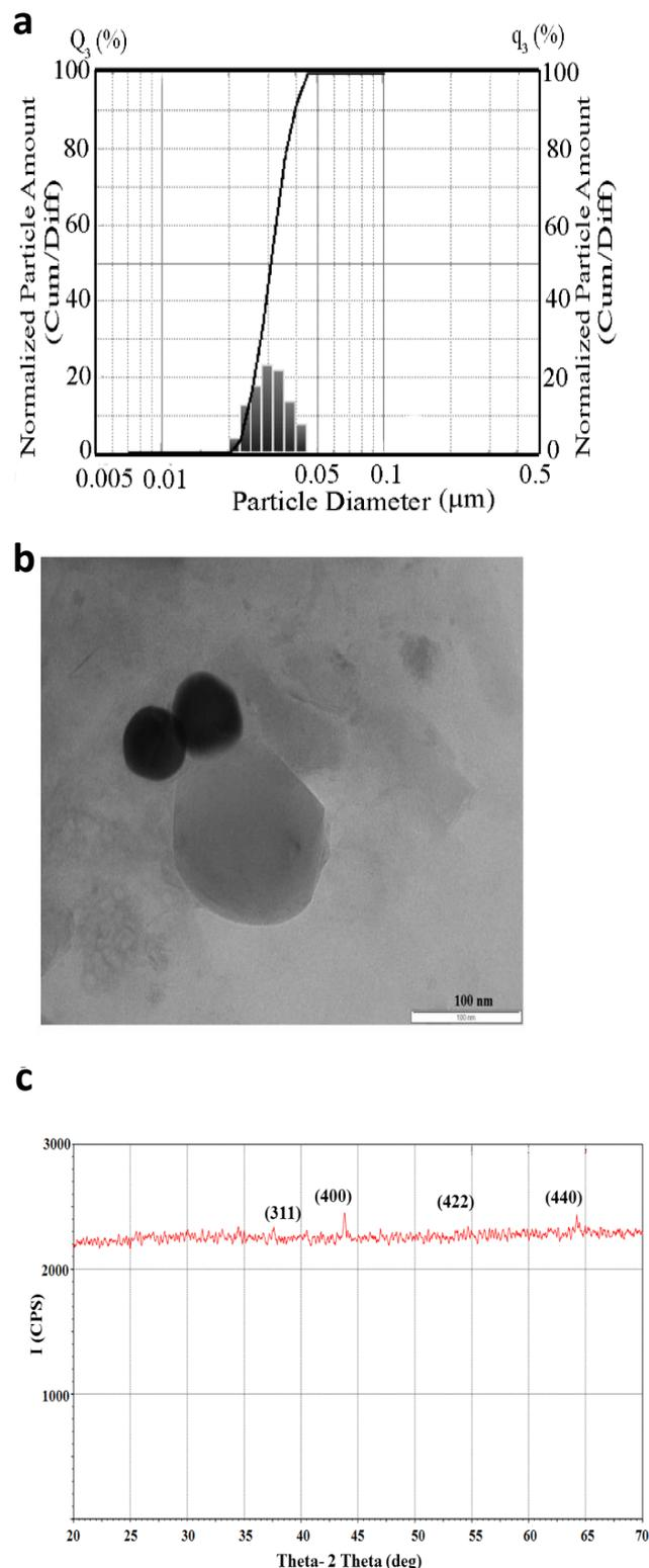
**Fig. 4** a. Particle size of MfeNPs. b. TEM image of MfeNPs c. XRD pattern of MfeNPs
