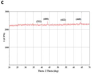
**Fig. 4 a**. Particle size of MfeNPs. **b**. TEM image of MfeNPs **c**. XRD pattern of MfeNPs
