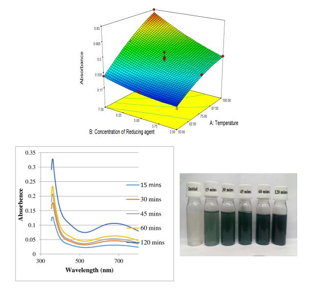
**Fig. 1** Response surface plot of Absorbance vs Temperature and concentration of reducing agent **Fig. 2** UV-Vis absorption spectrum of MFeNPs solutions at different time intervals. **Fig. 3** Images of MFeNPs solutions at different time intervals.
