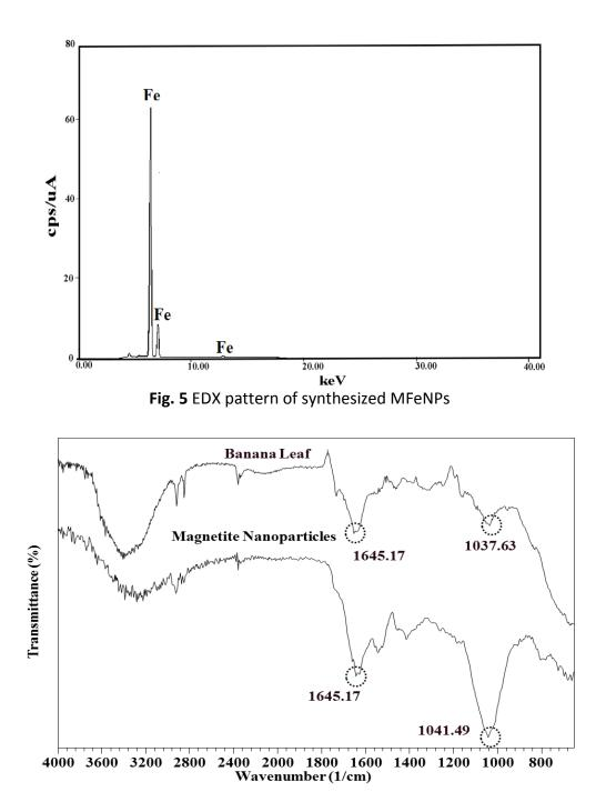
Fig. 6 FTIR spectrum of banana leaf and magnetite nanoparticles
